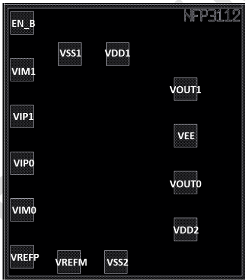
Figure 6 – Scale diagram of NFP3112 bare die pads. Overall dimensions are 1050 μm by 1200 μm
