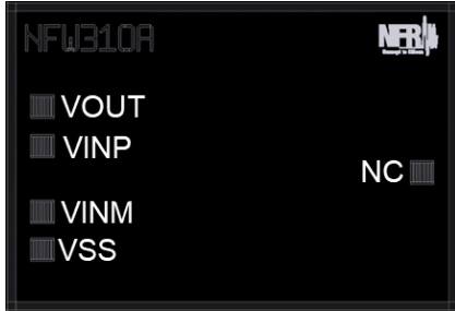
Figure 8 – Scale diagram of NFW310F. Overall dimensions are 850 \mu\text{m} by 580 \mu\text{m}
