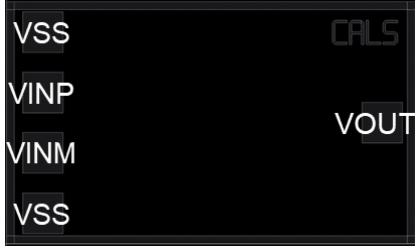
Figure 8 – Scale diagram of NFW310S. Overall dimensions are 850 \mu\text{m} by 500 \mu\text{m}
